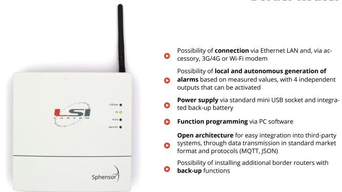
The primary function of the border router is to decode and route the radio messages arriving from the sensors via the Thread protocol to the MQTT broker reachable via the Ethernet connection and, vice versa, to send the messages coming from the same broker to the sensor or to all the sensors of the subnet. membership.
