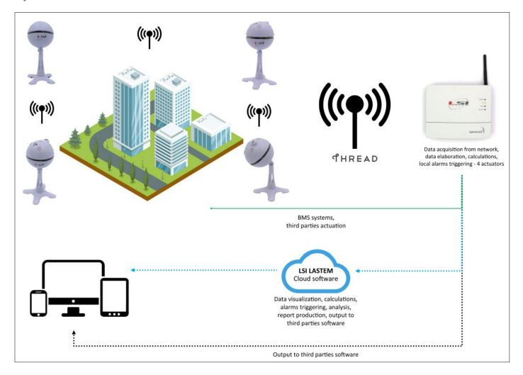
C The **Sphensor**<sup>™</sup> data logger sensors form an indoor sensor network and communicate with each other and with the border router via **2.4 GHz radio**, **Thread protocol**.
