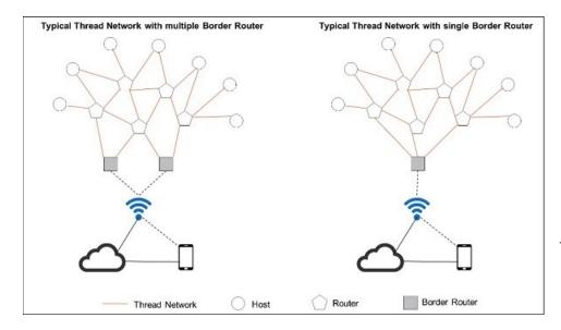
C The **Thread protocol** allows the connection and communication of the Sphensor<sup>™</sup> data logger sensor network to one or more border routers.
